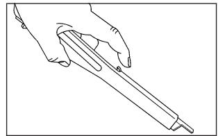
Extend the handle on the wheel wrench by pressing the button with your index finger and pulling on the end of the wrench. You must do this before using the wheel wrench.
